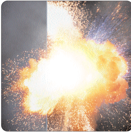
Arc flash explosions, like this one, are the result of a rapid release of energy due to an arcing fault between a phase bus bar and another phase bus bar, neutral or a ground.
