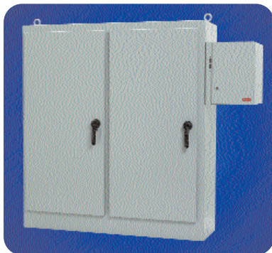
Hoffman's Sequestr External Disconnect Enclosure Isolates the switch in a small, interlocked enclosure so main power is no longer in the cabinet
