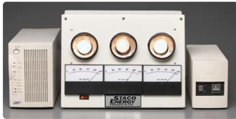
UPS system in a power swell situation
