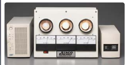
UPS system in a power sag situation
