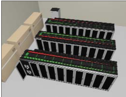
This graphic represents a data center layout in a hot-aisle/cold-aisle configuration with active heat removal rear doors that exhaust heat high up and close to the CRAC avoiding re-circulation.
