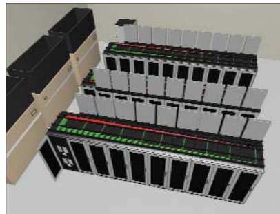
This graphic represents a data center layout in a hot-aisle/cold aisle configuration with active heat removal rear doors close-coupled with the return plenum through collars achieving double-digit kW heat removal.
